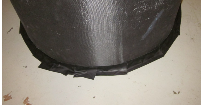
Figure 9.10 – Interface between the ground and the shell: tape and carpet ring for isolation.
