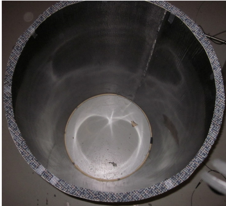
Figure 9.1 – Bare cylinder seen from the top. The isolating carpet ring is visible.
